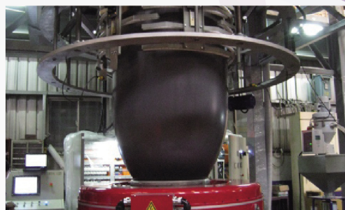
Automatic air ring for thickness control
