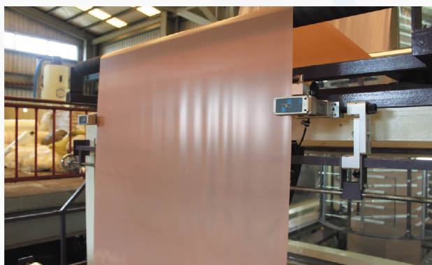
Central position control system
