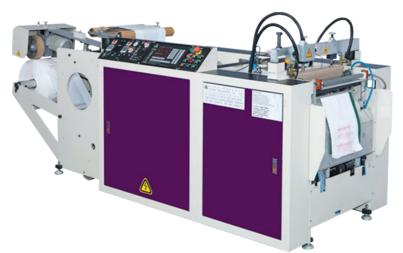
**MHSW** Hot Slitting & Sealing Re-tube & **Re-winding Machine**
